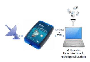
The use of an SDR transceiver is particularly elegant. This receives the IF signal from the LNB and transmits directly on the uplink frequency. It is usually connected to the PC by means of a USB cable. In the case of the ADALM Pluto, this can alternatively be done via an Ethernet connection.
