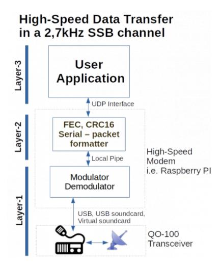
UDP ports are used as interfaces to the user program. This makes it easier for other developers to use the modem, offers independence from devices and operating systems and provides network capability.
