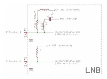
Modification of only one connector, which we select as we wish, but then permanently label it with WB so that it can also be easily recognized from the outside.
