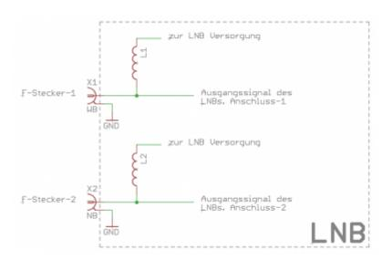
If you open an LNB, you can see the feed chokes L1 and L2 directly behind the connectors. These are printed directly on the circuit board as meander-shaped conductor tracks.
