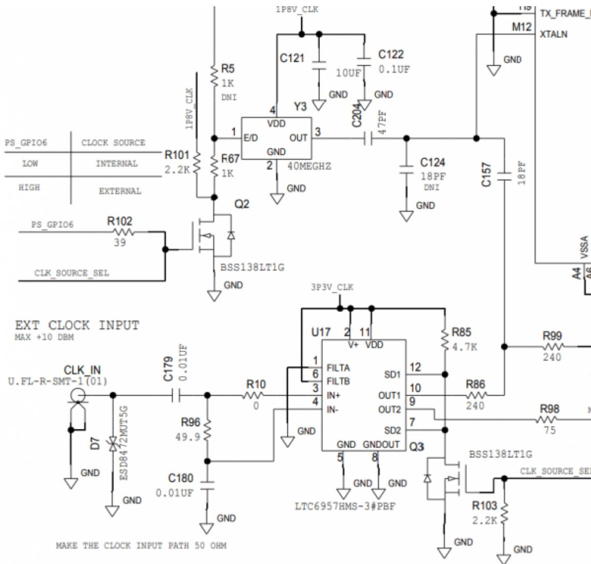
You can see that the ext. clock input is 50 ohms and there is also a DC block capacitor.
