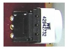
A 10-position switch allows selection of the output frequency. The display refers to the old frequency of the CW beacon. This was originally at 10489.550 MHz and was moved 50 kHz down to 10489.500 Mhz when the narrowband transponder was extended (from 250 kHz to 500 kHz).
