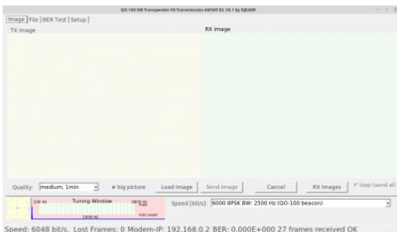
The IP address of the modem appears in the status line. If not, there is no network connection yet. As soon as the transceiver is switched on you can see noise in the constellation diagram on the lower left.
