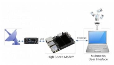
In this case you simply connect the modem and transceiver with a USB cable. In the picture the modem is running on an Odroid SBC. It can also run on the PC itself, in which case the single board computer fills and the transceiver is directly connected to the PC via USB.
