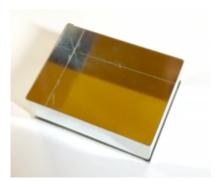
Using a hot soldering iron, solder the side panels (only the side panels, not the lid) so that a sturdy frame is formed.
