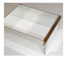
Insert the circuit board on a trial basis. The frame has a small protrusion on the inside, where the tinplate parts lie lie on top of each other. Use a file to file off the PCB at these two places so that it fits well into the tinplate frame. It is not soldered, just put it in on a trial basis. Now you can take the measurements for the connector cutouts. Cut (e.g. with a Dremel) or file three slots with 10 mm height and 6 mm width.
