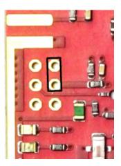
After connecting the 12 V supply line and possibly plugging jumpers for frequency selection, the lid of the tinplate housing can be put on. Finally, a label is glued on. The lid is not soldered, because you may have to make settings on the board (e.g. jumpers).
