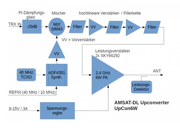
The 6-W output stage consists of two parallel SKY66292s. These, ICs built for cellular and wifi applications, provide high linearity with a gain of over 35 dB.
