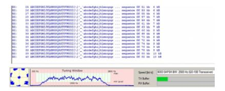
If all adjustments are properly done, "sequence OK" is always displayed. Error messages (frame lost) should occur very rarely. Of course, you can receive test data from other stations as well.
