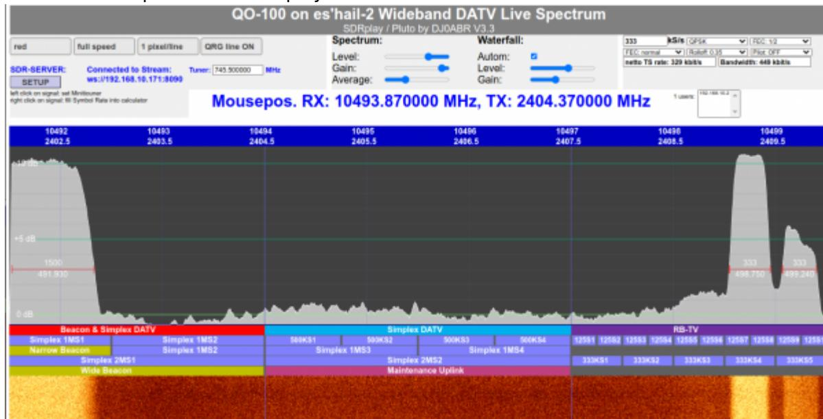
If you want to control a Minitiouner or a Ryde receiver, you fill in the corresponding fields in **SETUP**. Afterwards a mouse click into the spectrum is sufficient and the receiver is tuned to the frequency and symbol rate of the signal.
