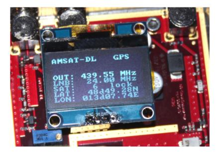
After the program start status information is displayed which correspond to the LEDs A to D. As soon as the system is synchronized the display shows frequency information, if the GPS module is mounted also GPS data.
