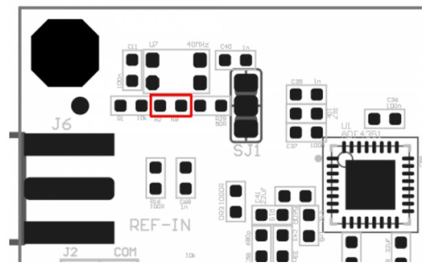
• If you want to be even more precise, you can install a 10kOhm 10-speed spindle trimmer from pin # 1 of the VCTCXO to ground instead of the 8.2kOhm resistor. For this you can use the left pad of R2 in the picture above. He can then set the frequency precisely at room temperature and only a small temperature drift remains.
