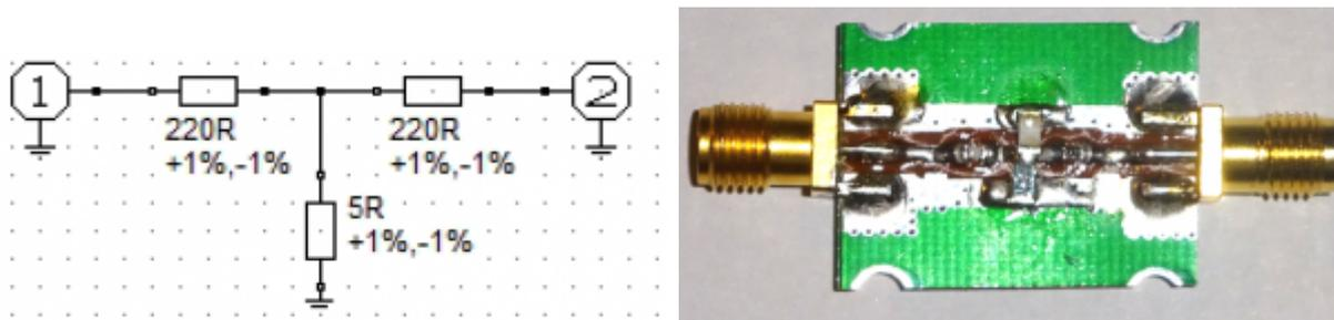
this attenuator has just under 40dB and deliberately no match to 50 ohms, because the focus here is on safety in case of accidental transmission, which would not be guaranteed with a 50-ohm
