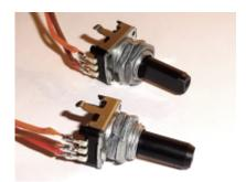
Rotary encoders have two internal switches with a common pin (usually the middle one), which is wired to GND. The two outer pins output a phase-shifted square wave signal when rotated which is applied to GPIO pins on the Raspberry header.
