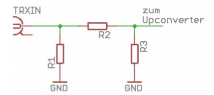
R1 must withstand the power of the transceiver and consists of two parallel 100 V resistors. Together with R2 (470 V) and R3 (51 V), this creates a 50 V attenuator with an attenuation of about 25 dB. Thus the upconverter can be driven with approx. 1 W (SSB). For special applications (e.g. driving with an SDR) this attenuator can be changed or removed completely. The driving power without attenuator should not exceed 5 mW.
